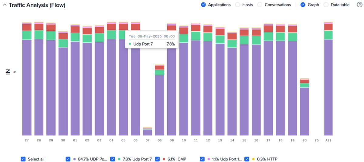
For fast identification of the causes of high utilisation, Flow in Highlight presents 10 minute granularity for the past hour, then smoothing data into hourly, daily and weekly summaries.
